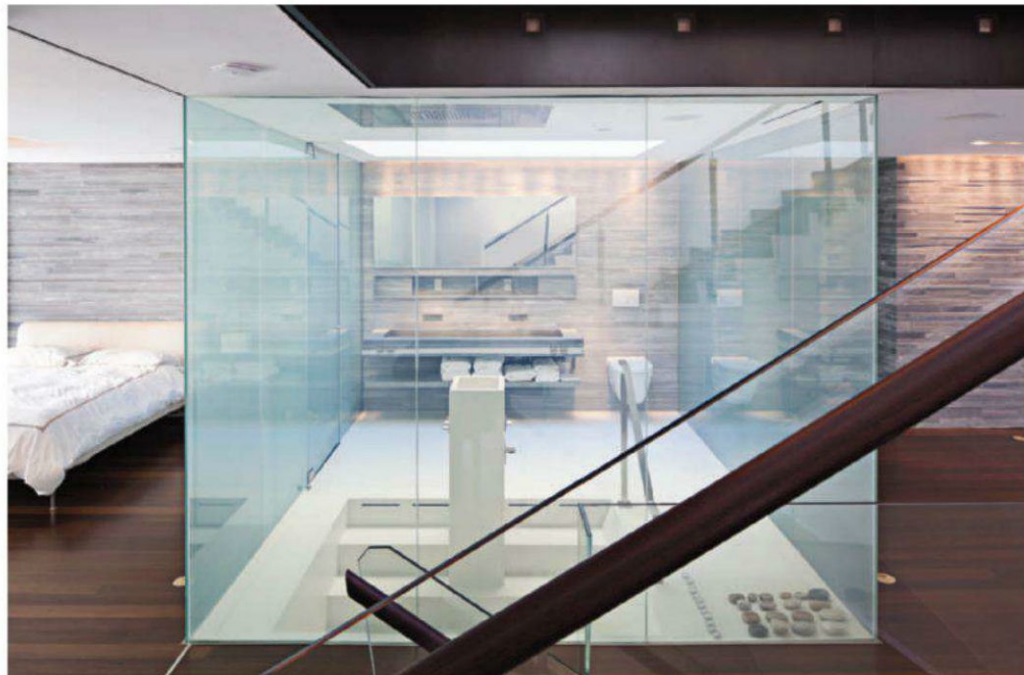
VANISHING ACT With the touch of a button, a low-level electric current runs between the panes of glass in the master bathroom to transform the walls from transparent (above) to opaque (right), allowing light in while retaining privacy.
