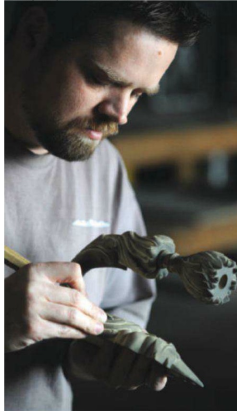
All bronze castings start with the creation of pattern by carving it out of wood or plastic.
