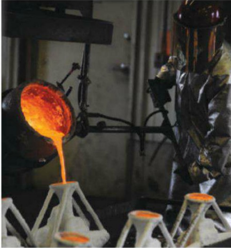
The completed ceramic molds receive the molten bronze and are broken away after the bronze cools to reveal the finished cast product.
