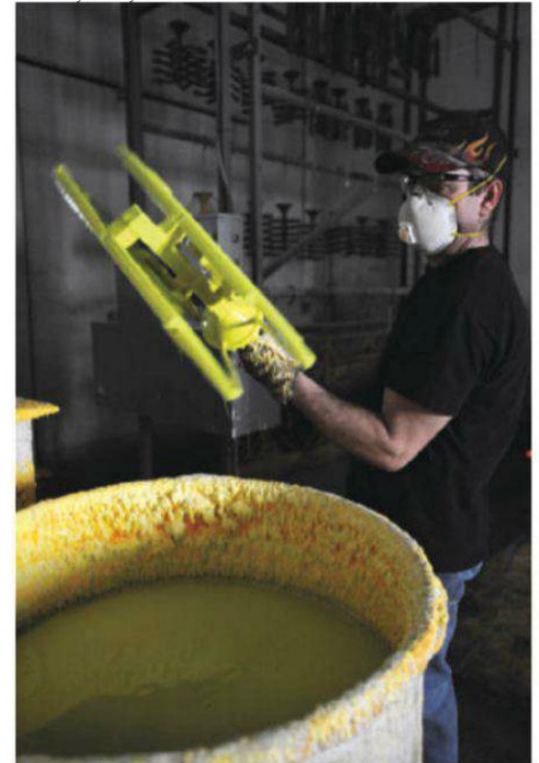
During the investment casting process, wax pieces are combined onto a “tree” of parts and dipped repeatedly into a ceramic slurry to create a ceramic mold.
