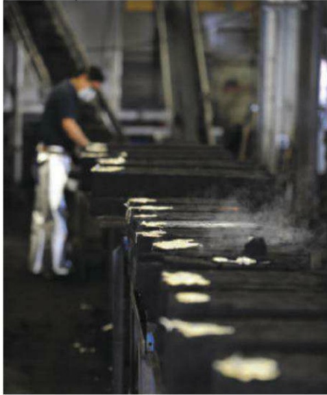
Sand molds are formed using pattern boards and then filled with molten bronze to create products using the common sand casting process.
