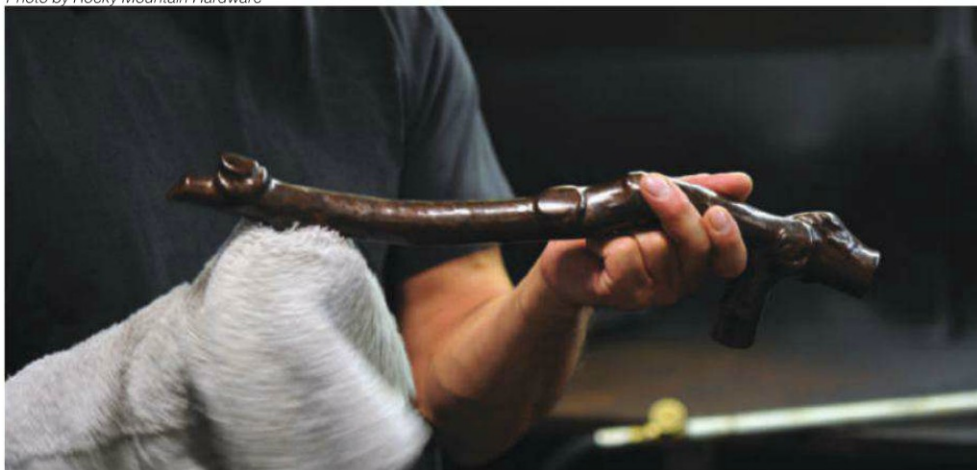
Cast pieces are finished and polished by hand.
