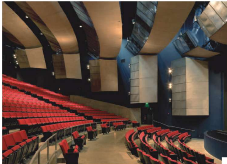
1. The theater has acoustic "clouds" overhead, a full orchestra pit, a 30-student tech booth, and 32 drops in the stage floor. 2. the diagonal steel structure is revealed in the dance studios, as
