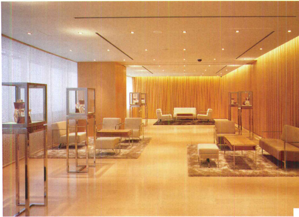
1,3. Within the shop, the architect and lighting designer specified space-saving LED tape to accommodate building constraints, halogen spots for sparkle, and fluorescent fixtures for ambient illumination.
