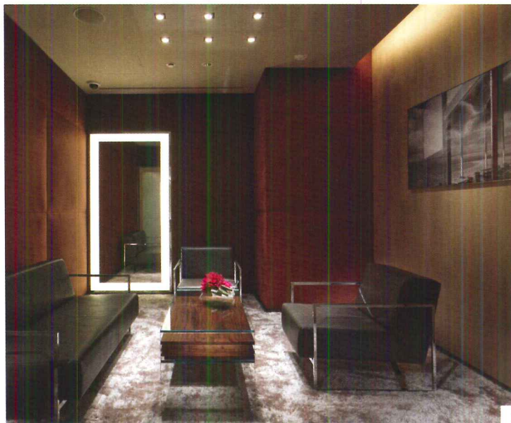
1,3. Within the shop, the architect and lighting designer specified space-saving LED tape to accommodate building constraints, halogen spots for sparkle, and fluorescent fixtures for ambient illumination.
