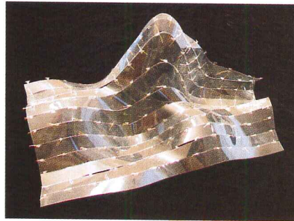
Lamina aids the design and production of complex 3D forms made from planar materials like metal and wood.
