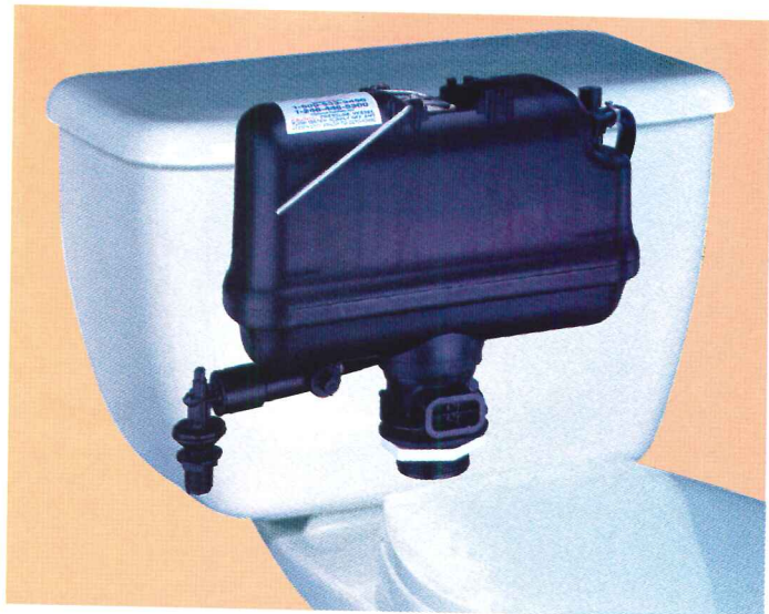
The FlushMate IV pressure-assist toilet flush mechanism features an inner airtight flushometer tank that is pressured after the flush as the tank refills. During the flush operation, this air pressure flushes the toilet with increased velocity, improving flush performance. Sloan Valve, Franklin Park, Ill. www.sloanvalve.com CIRCLE 210
