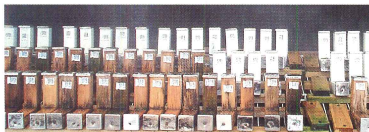
Top: L-joints during exposure in Hilo with differences in mold on paint. Bottom: Greenhouse setup of L-joints for artificial spraying of water.
