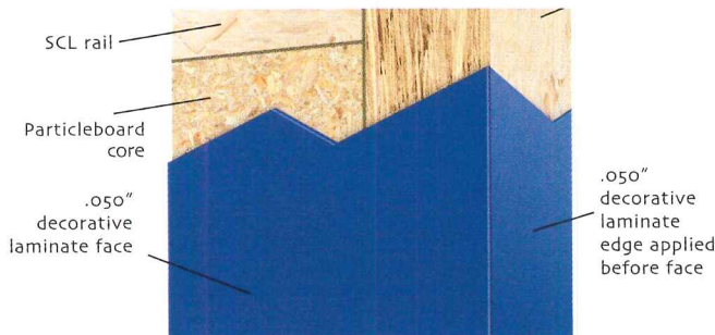
It is possible to purchase decorative laminate doors with the laminate edges applied before the face material, which protects the edges from peeling, chipping, or breaking.
