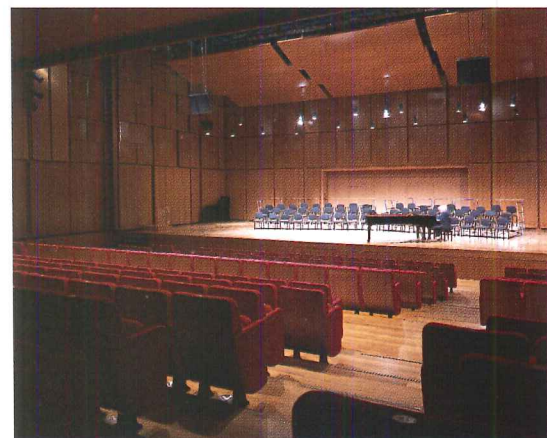
The two smaller concert halls (above and left) are highly flexible acoustically, with adjustable cherry ceiling and wall panels. But the most elaborate acoustic forms belong to the symphony hall (top), where 26 ceiling hulls are sized and shaped to disperse sound and resolve echoes.
