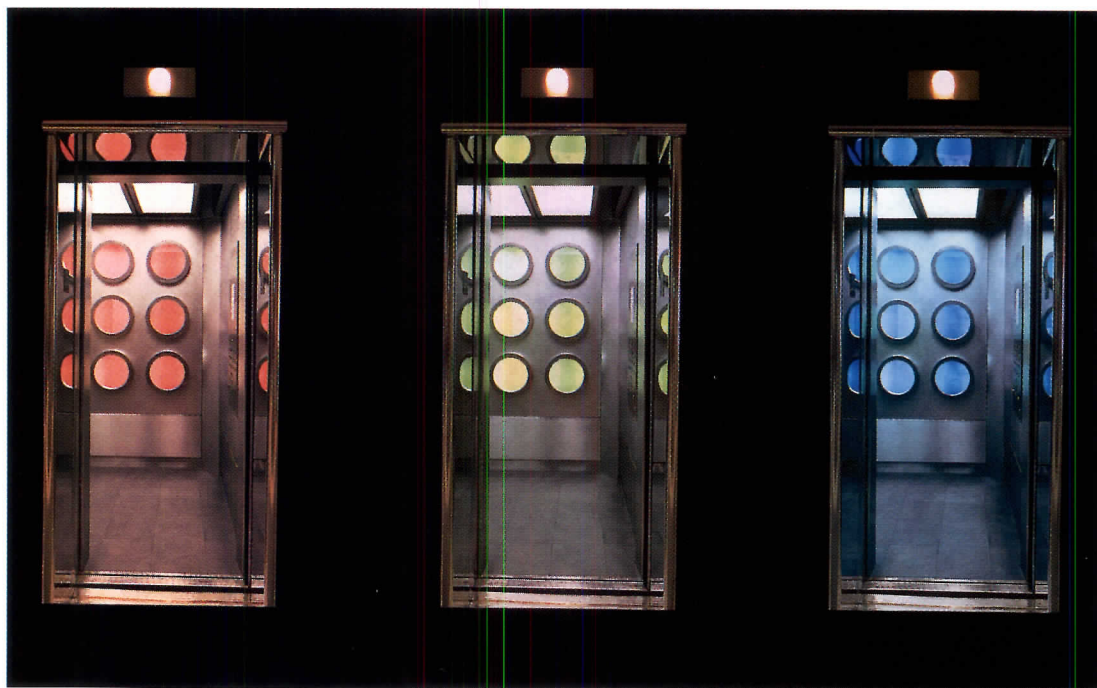
Dichroic filters backlit by fiber optics decorate the elevators in Color Wheel's office building in midtown Manhattan. The colors represent the basic red, green, and blue used in the firm's printing and computer-graphics work.
