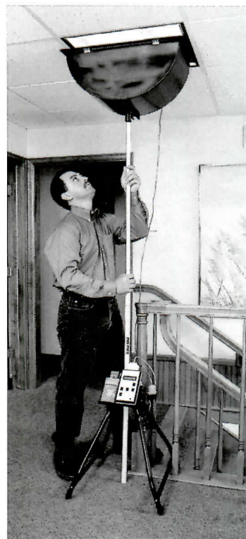
In a new luminaire dirt depreciation study, light output was measured before and after fixtures were cleaned.
