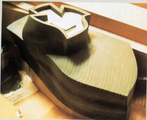
A COMPUTER-CUT MILLED MODEL IS MADE TO VERIFY ACCURACY
