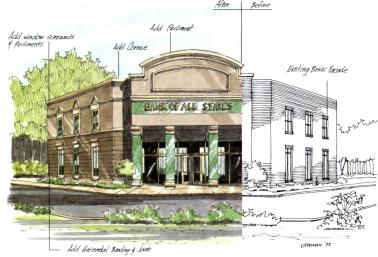
GIVE A UNIFIED LOOK TO DIFFERENT, ATTACHED BUILDINGS. SYSTEM SHOULD NOT SHOW CONTROL JOINTS. VARIETY AND CONDITION OF EXISTING WALLS MANDATE
