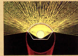
A selection of specially-designed lenses distributes light facet by facet. This up light combines wide spread with low lens brightness.
