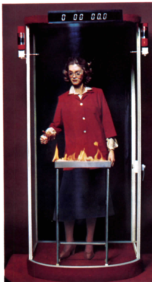
1. Flammable liquid ignited. Halon 1301 cylinders discharged.
