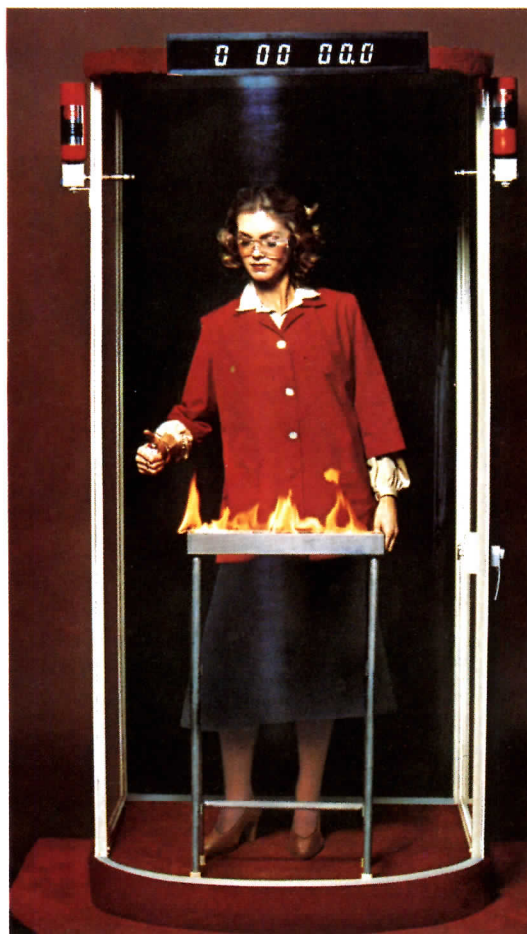
1. Flammable liquid ignited. Halon 1301 cylinders discharged.
