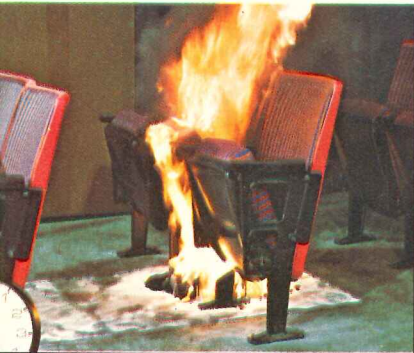
TEST TWO: HR POLYURETHANE containing flame retardants. Time: 1 minute, 30 seconds after ignition.
