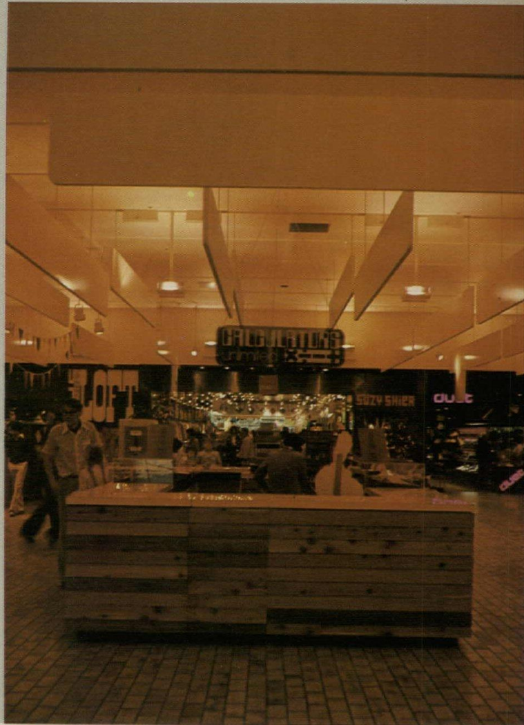
Special-profile luminaires direct light within narrow angles to illuminate broad areas of structural framing in the high-bay areas and ceilings of the strip mall.
