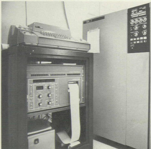
Data from a weather station and from instrumented equipment in the Bridgers and Paxton building is acquired by computer and sent to Penn State for analysis.
