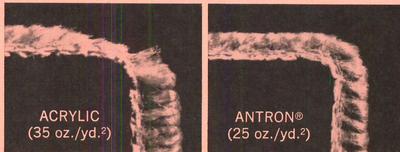
Abrasion test of simulated stair edges showing carpet pile fiber wear in level-loop carpets after equal exposure.
