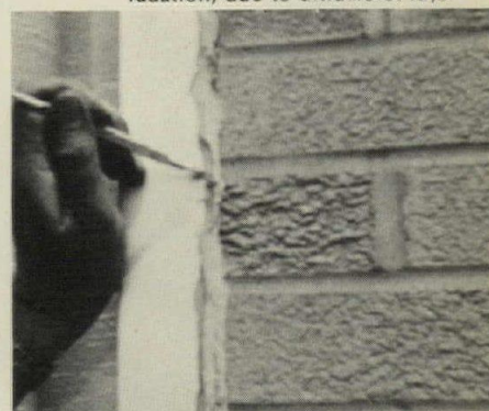
Sealant never set up—probably the result of improper formulation Below: Examples of sag (vertical joint) and weep (horizontal joint) caused by faulty compounding
