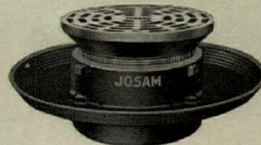
No. 300-A-SF Floor Drain with Super-Flo strainer for kitchen and shower areas. Greater strainer free area increases flow through drain. Perimeter slots permit water to keep drain clean.
