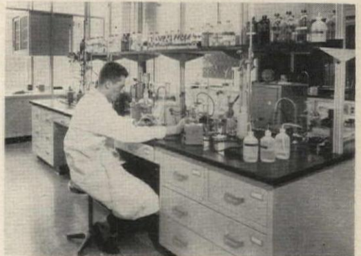
While most of the work benches are 37 in. high, those requiring sit-down operations, as shown here, are 31 in. high, with knee space provided for the operator. Vertical channels at back of lab benches provide adjustable supports for shelves and for equipment. All steel cabinets have a bonderized epoxy finish so as to withstand concentrated reagents
