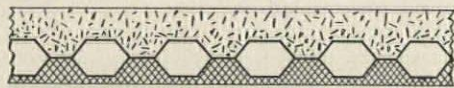
4 hours fire protection for this standard cellular steel floor unit required only a \frac{1}{2} " minimum thickness of SPRAYED "LIMPET" ASBESTOS below the steel.
