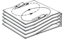
When the ramps are separated, new circulation schemes are possible. This one has opposing circulation and two points per floor where the paths must cross culation will be important. The garage will have to load up in a hurry at 8:45 to 9:00 AM and empty quickly at 5:00 PM.
