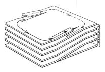
The circulation is more logical with this arrangement. It is the most straightforward ramp system
