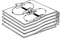
In this arrangement, the circulation has been completely separated. This is the most straightforward of the staggered floor systems
