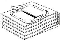
This simplest of staggered floor systems has the obvious fault of opposed circulation. In all of these staggered floor schemes one floor may be narrowed to mezzanine size
