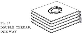
Ramps are steeper since they only have 180 deg to get between floors. A popular design with separated flow
