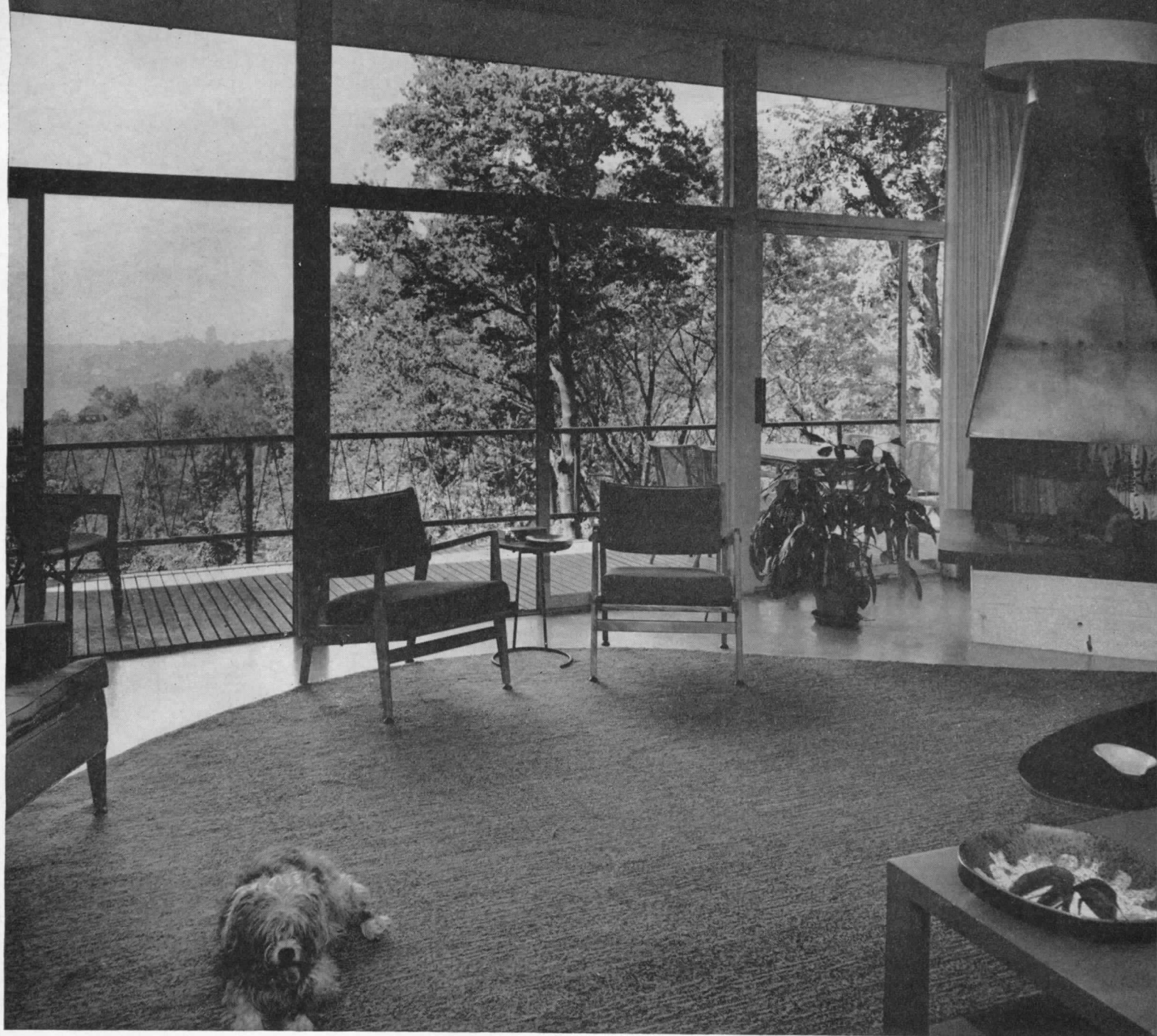
Structure. Concrete block, concrete footings and piers; wood frame; exterior walls, redwood; floors, asphalt tile over plywood; plaster ceilings. Free-standing fireplace resulted from owners' desire for fireplace on view side without spoiling view. Roof is built-up with gravel and oyster shells
