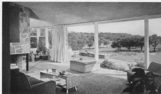
Site Relationship. Site is large, with a long gradual slope at rear which low pitch of roof echoes; living room has floor-to-ceiling glass wall which extends room to far corner of site. Materials. Vertical T&G siding and painted (red) plywood panels on exterior; concrete floors
