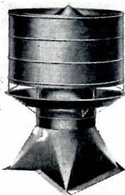
American Blower upblast type exhaust ventilator exhausts corrosive, oil- or grease-laden fumes at high velocities. Housing: Heavy-gauge welded steel, phosphatized for rust resistance; baked enamel finish Stack Cross Section: 32 \frac{1}{4} " to 56 \frac{3}{8} " Capacity: 7600 to 34,500 cfm Mfr: American Blower Corp., Detroit 23, Mich.
