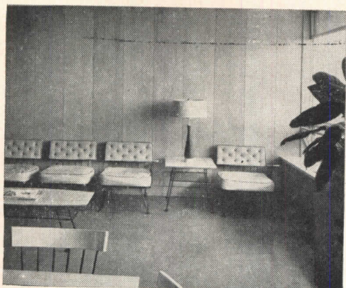
EASY-TO-INSTALL OAK PLANKWELD adds a cheery note to this waiting room. Plankweld can be installed on any wall with special metal clips which hide nails.
