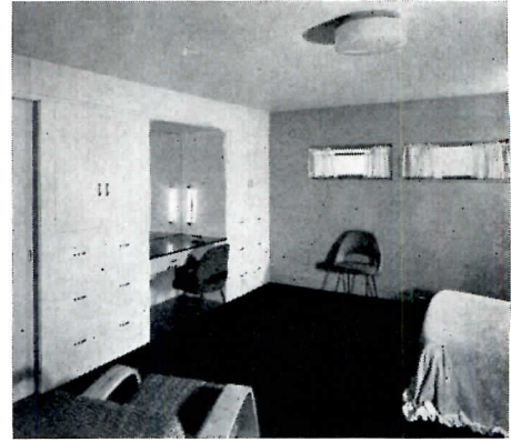
Storage walls in bedrooms form sound barrier against living room. High windows in master bedroom help ventilation, privacy
