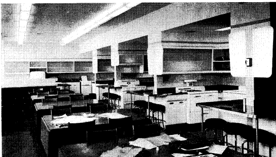
Each classroom is designed for a special purpose. All have painted concrete block walls, acoustic tile ceilings, asphalt tile floors, aluminum sash, fluorescent light, finned radiation, unit ventilators, blue glass chalkboards. Right, top to bottom: social science room; home economics laboratory with demonstration area at far end set off by low tiled wall; drafting room; general shop whose beamed ceiling, formed by concrete pan construction, accommodates fluorescent light strips
