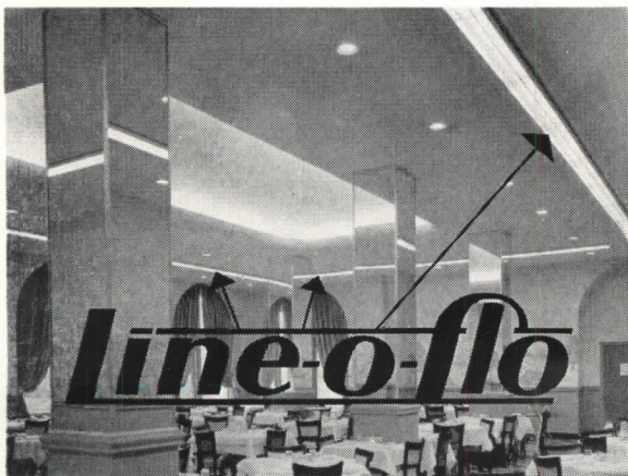
Illustration of continuous-strip "LL" LINE-O-FLO units with lights in the ceiling of a hotel dining room.
