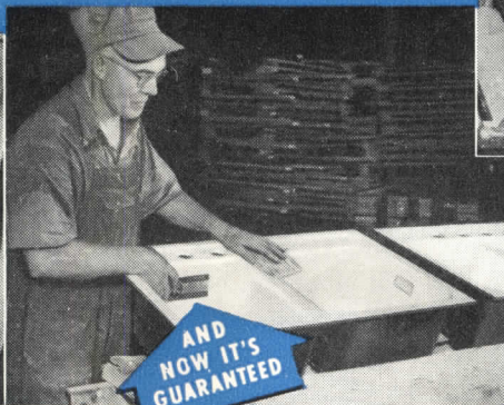
Edward Roth, 37 years an enamer, critically inspects his handiwork after he has applied the Richmond Whiter-white enamel to the sink casting.
