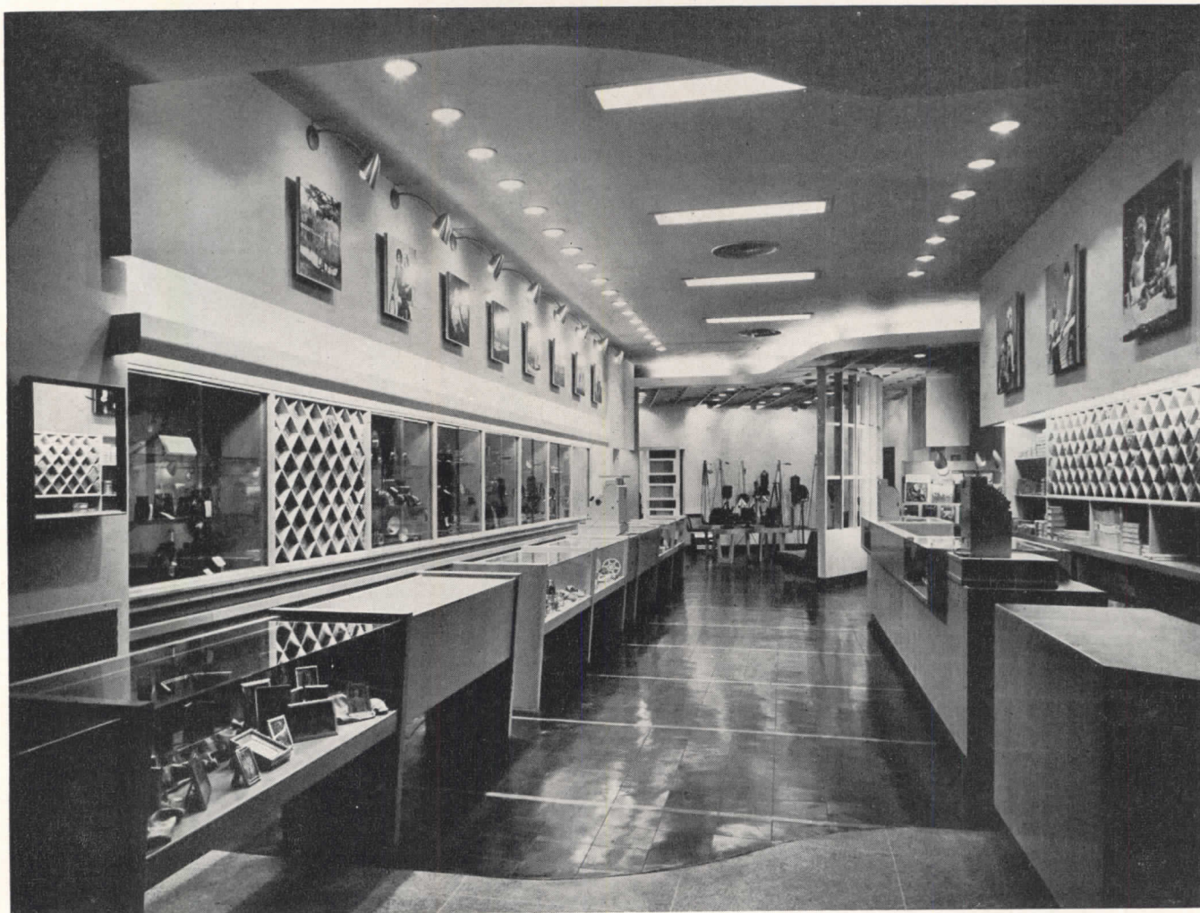
Store front is of gray structural glass, vestibule ceiling is plaster painted pale yellow. Interior woodwork is pickled oak, wall above cases is sea green and ceiling is pearl gray. Main flooring is black asphalt with deep green strips inset
