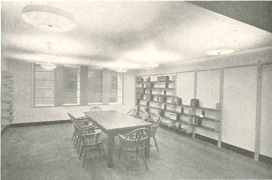
Above (3): Bay set up as model departmental conference or seminar room. Wall shelves will contain books used continuously in departmental operations. Experimental flooring here is half random wood plank, half parquet squares. General type and effect of lighting equipment in this bay were favored by library planning committee (see text)
