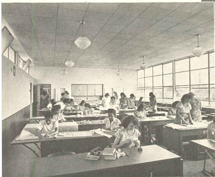
Sewing-room view below shows how well bilateral lighting works in the classroom width of 26 ft. 6 in.; and the view (right) taken at the front of the same room shows the orderliness of well-designed, cleanly carpentered cabinets finished in birch plywood (note the triple suspended blackboard). Classroom walls are plaster above 3-ft. natural birch wainscot; ceilings acoustic tile, floors asphalt tile. At left, rear, in the classroom view a girl is seen using the triple mirror in a carefully equipped fitting room
