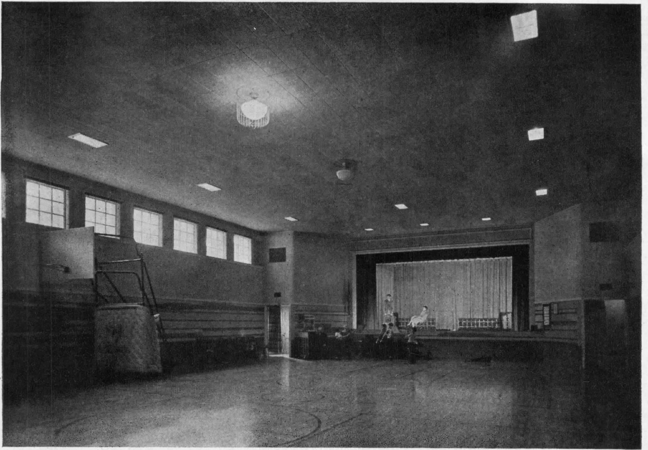
The auditorium is larger than customary for this type of school because it serves not only for the usual school purposes but also for dramatics and community activities. The maple flooring is laid on wood sleepers
