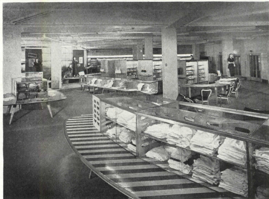
"Upside down" tables eliminating the separate sales person's aisle; applicable also to self-service. Note fluid arrangement of department in rear, permitting access to high storage units for all sales peoples allowing easy change in relative front devoted to different kinds of goods. (Kauffman's, Pittsburgh, Kenneth C. Welch, consulting architect, John Schurko, designer)
