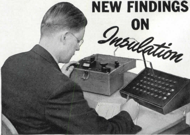
Taking temperature readings at 43 thermocouples with potentiometer.
