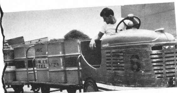
SEGREGATION MINIMIZES SCRAP LOSS —A western aircraft plant has more than doubled its scrap collections through a systematic salvage program, directed from a central office. All metal scrap is segregated into solids and machinings, and also by alloy content, right at the machines. Scrap containers are color-banded and labeled to clearly identify what goes into each . . . Have you organized an efficient scrap collection system at your plant? Does it provide for careful segregation?
