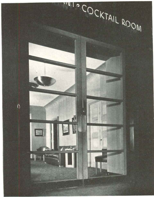
No. 1: From a station entrance, the door leads into No. 2: the carpeted foyer. Walls, white-oak veneer on flexible backing
