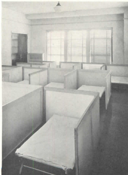
Venetian blinds are used to dim natural light; artificial lighting fixtures are semi-direct; sleeping room, Cornell Nursery School
