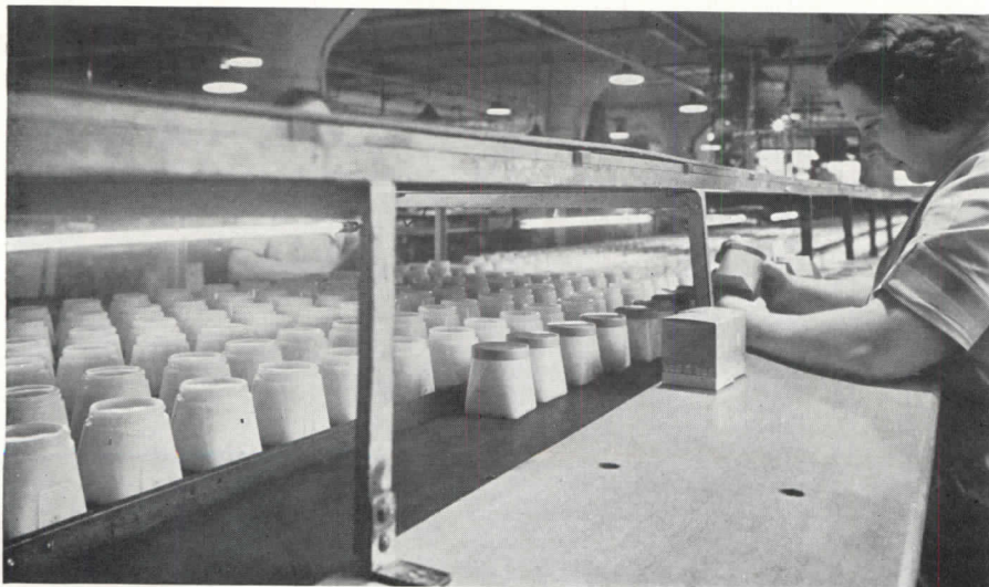
INDUSTRY: In this cosmetic factory, jars are passed under a bank of Sterilamps for sterilization while cooling.
