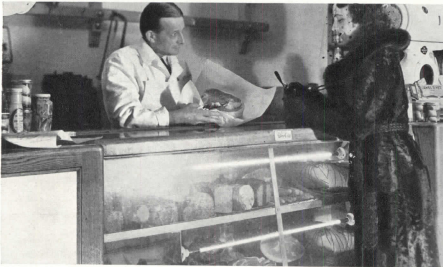
MEAT MARKETS: Meat can safely be stored at much higher temperatures either by direct application of Sterilamp (above) or in sterile air.
