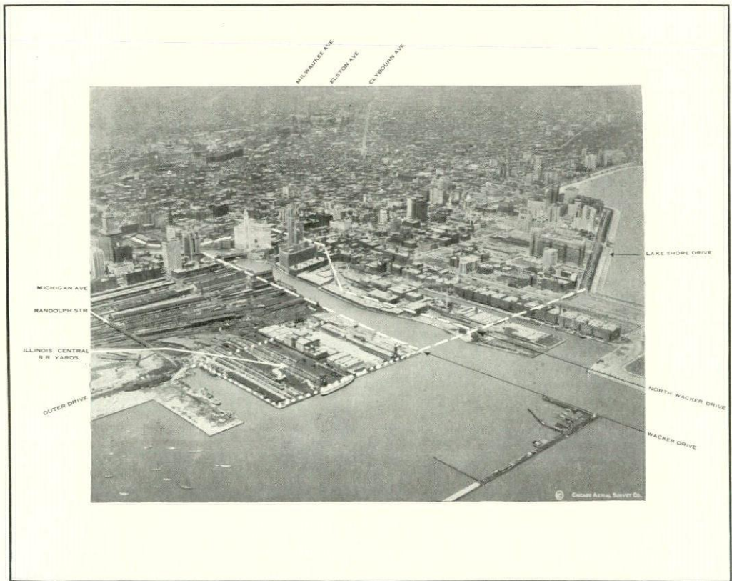
Aeroplane view which shows the proposed extension of Wacker Drive east to Lake Michigan and the proposed parallel drive along the north bank of Chicago River; also the contemplated link between the Outer Drive (which now ends at Randolph Street), and Lake Shore Drive. Dotted lines show extension of Outer Drive directly north to Wacker Drive and the alternative plan under consideration which involves the extension of Randolph Street to the lake
