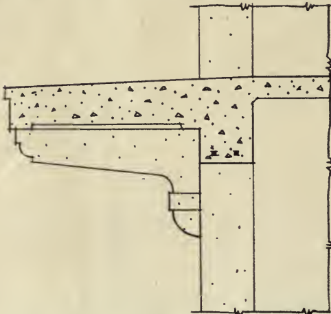
FIG. 12. BRACKET DETAIL IN CONCRETE.
