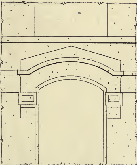
FIG. 10. DESIGN FOR DOORWAY TREATMENT IN CONCRETE.
